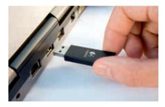
5. Plug the receiver from the cordless pointer into the laptop and switch on the pointer.
