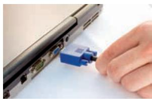
2. Plug the cable from the PC projector, or other external display device, into the matching port on the laptop. Switch on the external display device and switch on the laptop.
