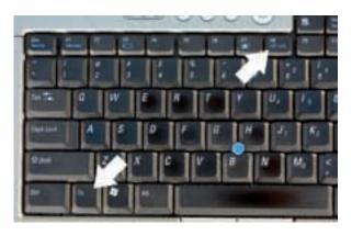
3. The laptop may detect automatically the external device. If not, on most laptops one uses the 'Fn' key and a key marked 'CRT/LCD' (and/or with a little picture of a monitor) to turn the display on manually.
