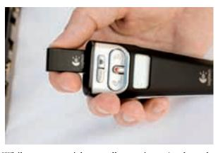
4. While not essential, a cordless pointer (such as the Logitech<sup>®</sup> shown here) is useful for controlling the presentation while standing or walking around. The main button advances the PowerPoint<sup>®</sup> slides.
